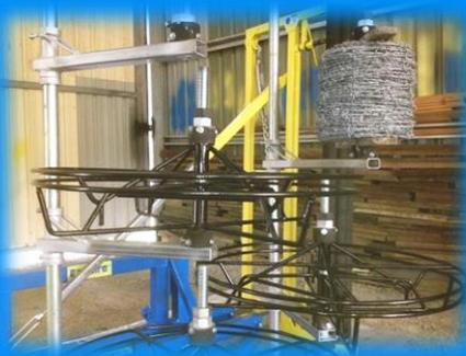
Multiple plain wire spinners and barb spools can be handled on elbows that fit onto the wire roll shafts. These elbows have a braking system that stops overrun of the wire. If necessary the **Ezywire™** can be detached and chained to a post or pegged down to the ground and the vehicle (tractor/bobcat etc.) can pull out multiple wires in one pass, such as when wire is pulled through split posts or in places a tractor cannot get.
